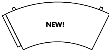
96-9201-L/CI-8201-L High Line Longer Curved Left Arm Facing Section Outside L89 D42¾ H33 Inside L75¾ D22¼ Seat H18 Arm H22¼
